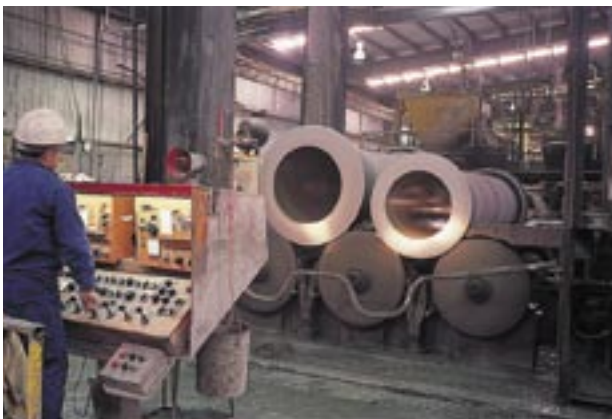
The manufacture of centrifugally spun pipes.
