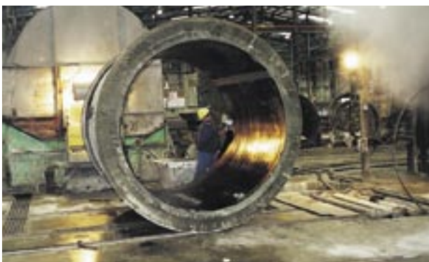
Plastiline™ installed in pipe at moulding stage.
