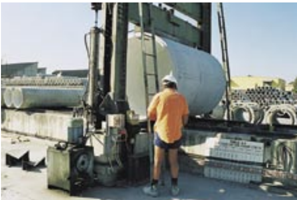
Routine testing of pipes to validate Load Class compliance.
