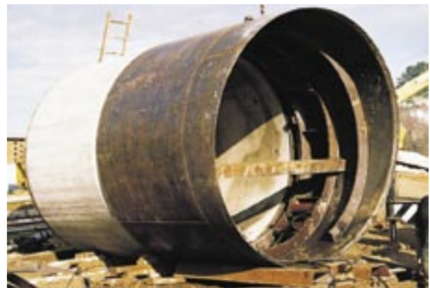
Jacking shield on lead pipe.
