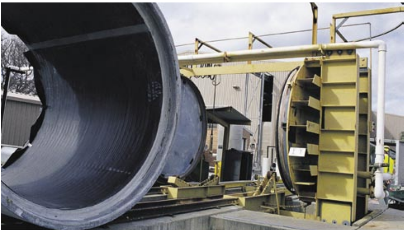
Routine Hydrostatic testing of 2250mm diameter Plastiline™ pipes at Humes Welshpool Plant in Western Australia.
