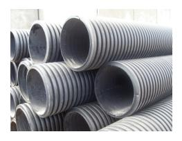
The smooth inner wall surface provides excellent hydraulic flow capacity. It is also resistant to abrasion, corrosion and chemical scouring. The ribbed outer wall provides optimum strength and has the ability to support heavy loading. This form of flexible pipe has the ability to relax under stress which reduces the possibility of damage.
