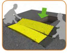
8. Lower next plate at an angle so the connectors fit into the slots.
