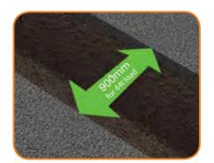
**1.** Ensure max trench width less than 900mm for 44t load, and less than 1200mm for pedestrian load.
