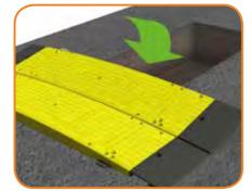
9. When the connectors are in the slots carefully lower the plate.
