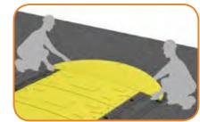
2. Starting from the end sections, carefully lift the plate at an angle and slide outwards to remove plate.
