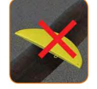
13. End section should not be placed over the trench.
