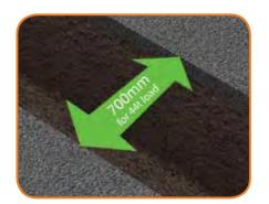
**1.** Ensure max trench width less than 700mm for a 44T load. Assess trench stability prior to install.
